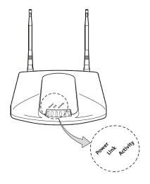
Power Flashing indicates AP initialization. Shows steady green during operation.
